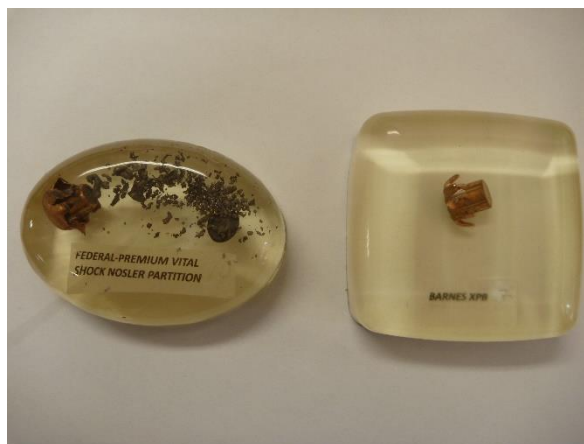
Figure 6: Lead (left) versus non-lead (right) ammunition after mass retention testing conducted by the Yurok Tribe.
